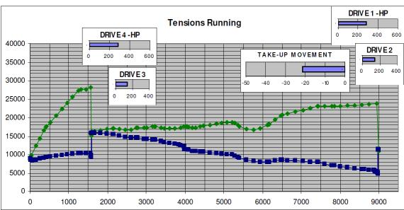
Real time analysis quickly reveals the tension and power distribution due to various material flow conditions at overland conveyor.
