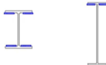
Figure 2: Examples of Structural Reinforcements
