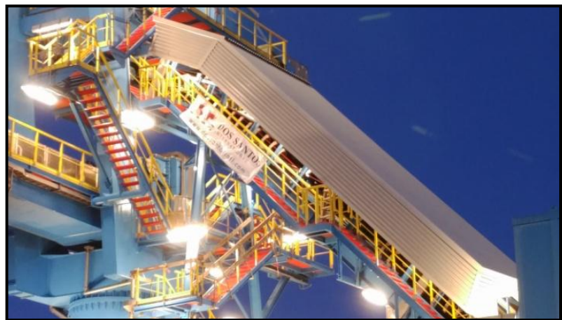
Figure 2: DSI Sandwich Conveyor with Adder
