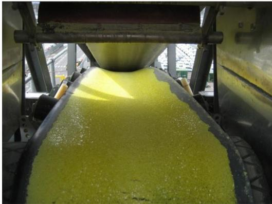
The Oxbow Sulfur Handling facility takes in liquid sulfur which is turned into pastilles using a steel belt system. From the steel belts, the material must be transferred into a silo. The pastilles are then loaded into trucks for export. The challenges the customer had were the need for a system fitting into a small footprint, total utilization of the money making materials, more efficient containment of materials and cost savings advantages.
