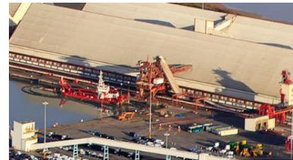
Figure 2: Sandwich Conveyor fed by low-lift tripper
