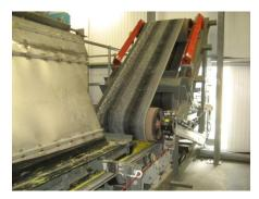
DSI developed the Semi-Automatic Take-Up initially for use on the smaller variations of the DSI Sandwich belt high angle conveyor. Consistent tensions are extremely important on these units, and these are typically maintained by hydraulic take-up units. With smaller units however, it made sense to develop a solution which would incorporate the manual take-ups more suited to short centered conveyors.
