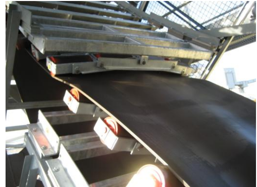
FEI's (Fully Equalized Idlers) at the inflection zones ensure continuity of hugging regardless of the conveying rate.
